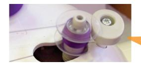
5 Put your foot on the pedal & watch the thread wind around the bobbin!
