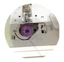
Check the bobbin. If there is thread on it like this picture, skip to PART 2. If there is no thread, you are going to need to WIND THE BOBBIN.
